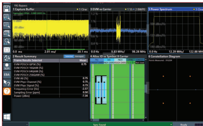
▲ Fig. 1 Screenshot of a measured 5G NR signal at 28 GHz with EVM below 1 percent.
